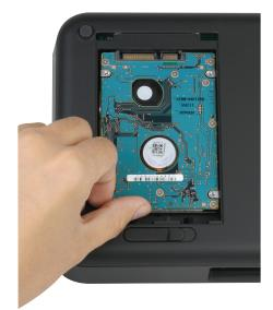
Place the bracket over the hard drive as shown, and secure the hard drive with the included screws. Replace the hard drive cover and slide the drive lock to the locked position.
